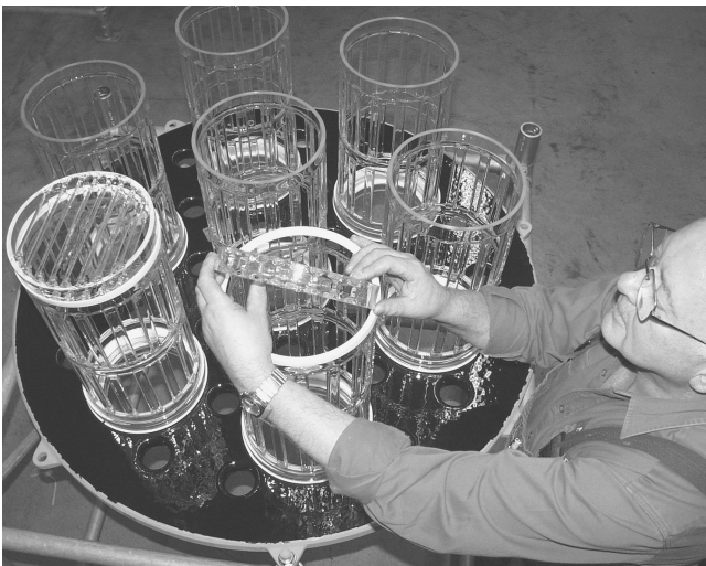
Fig. 1: CORE-TRAY DN 1000 assembly, here for packing with glass support
